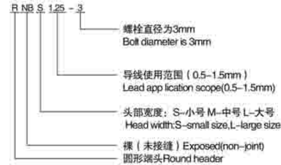
冷压接端头型号及其含义 Could press-connection header type and its meaning
